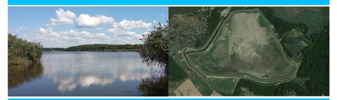
The Pearce Creek Dredged Material Containment Facility (DMCF) was reactivated to receive dredged material in 2017 after installation of an impermeable liner.
